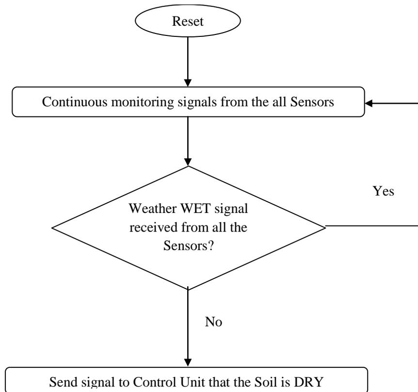
*Fig.2 Working of Moisture Sensing Unit.*
