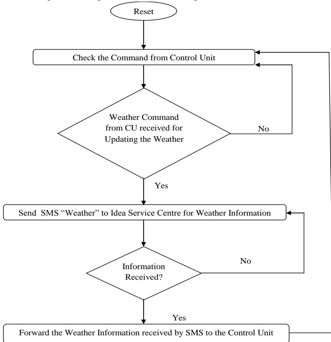
Fig.4 Working of Weather Forecasting Unit
