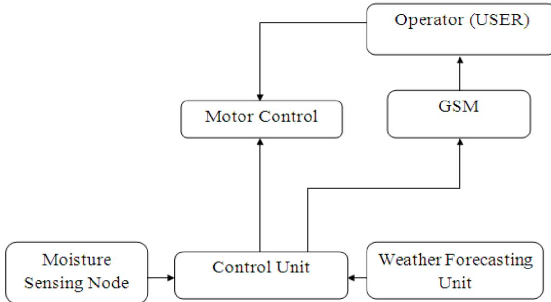
*Fig.1 Block diagram of WSN and Weather Forecast Based Irrigation Regulator System*
