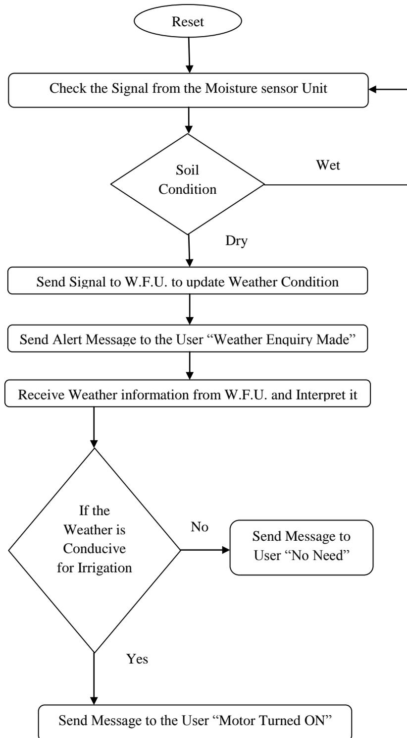
**Fig.3 Working of Control Unit**
