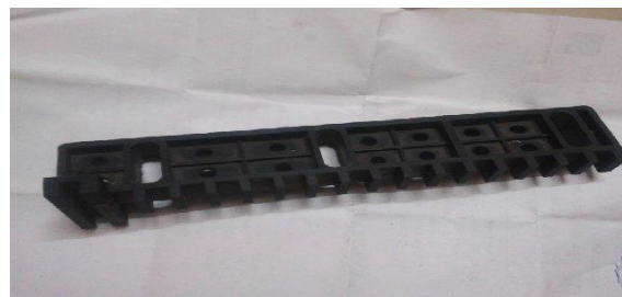
Figure: 1.4 Slider connector in water jet looms.
