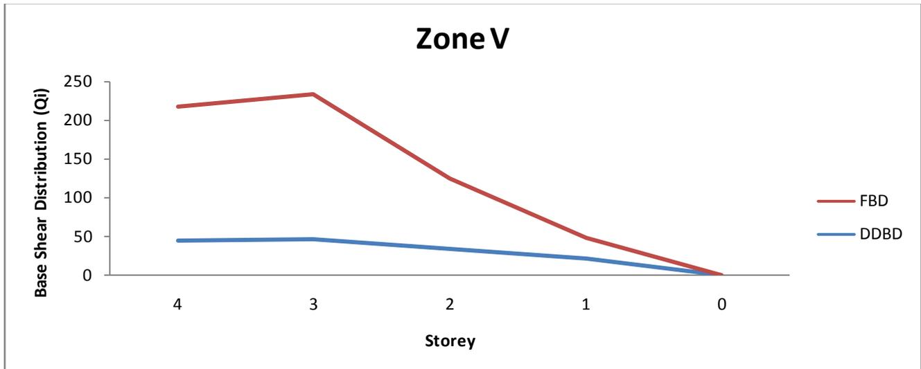
Figure 6 Graph of Base Shear Distribution for Zone V
