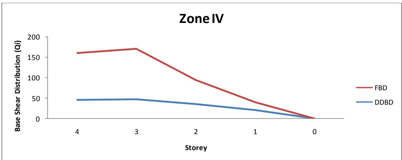
Figure 5 Graph of Base Shear Distribution for Zone IV
