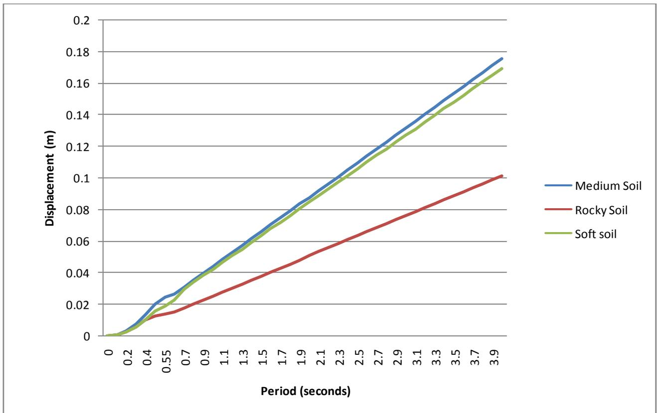
**Figure 2: Response Spectra for 5% damping [IS 1893 (Part 1) 2002]**
