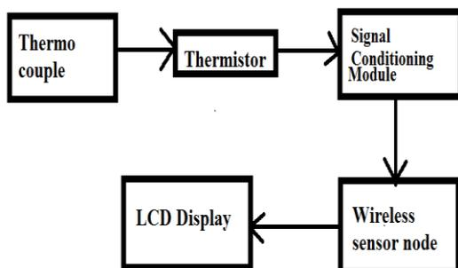
**Fig.1 The block diagram for powering a wireless sensor node using thermal energy .**
