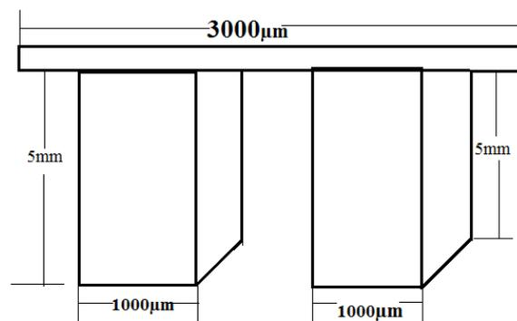
**Fig. 2 Thermocouple model with dimensions of left leg, right leg and connector.**
