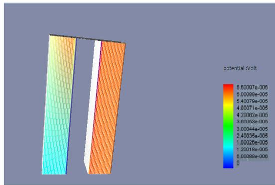
**Fig 7 Potential distribution of thermocouple obtained in Thermo electric module in intellisuit software.**
