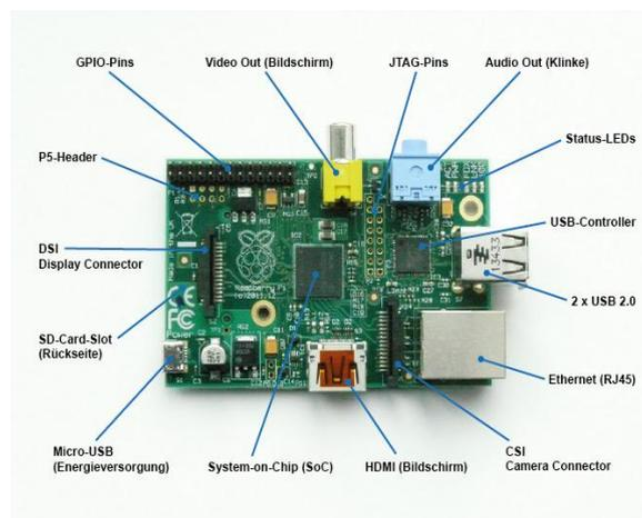
**Figure 1. Raspberry Pi Model B**
