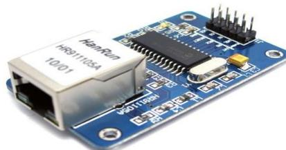
*Figure 7. Ethernet Module (Enc28j60)*
