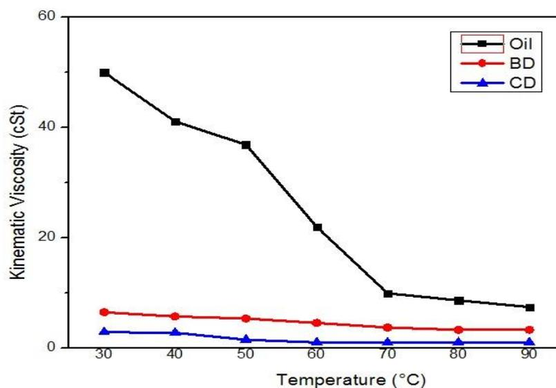
Figure 4. Comparison of kinematic viscosities of rubberseed oil, biodiesel and diesel inrelationship with temperature.
