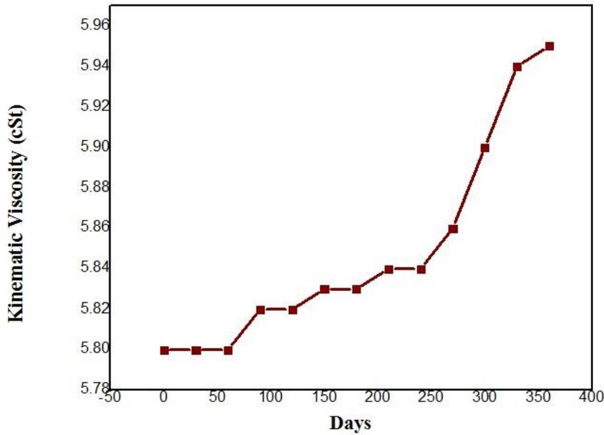
*Figure 7. Changes in kinematic viscosity of biodiesel during storage.*
