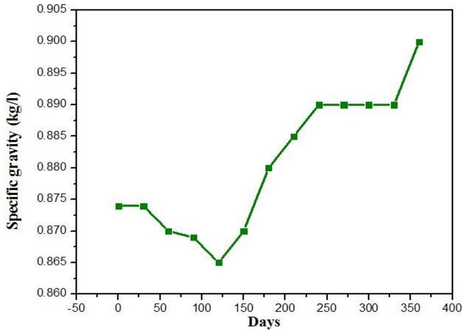
Figure 5. Changes in specific gravity of biodiesel during storage
