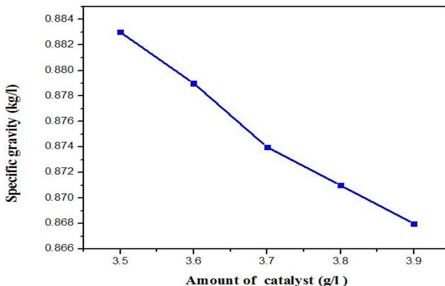
Figure 3. Effect of specific gravity with respect to catalyst.
