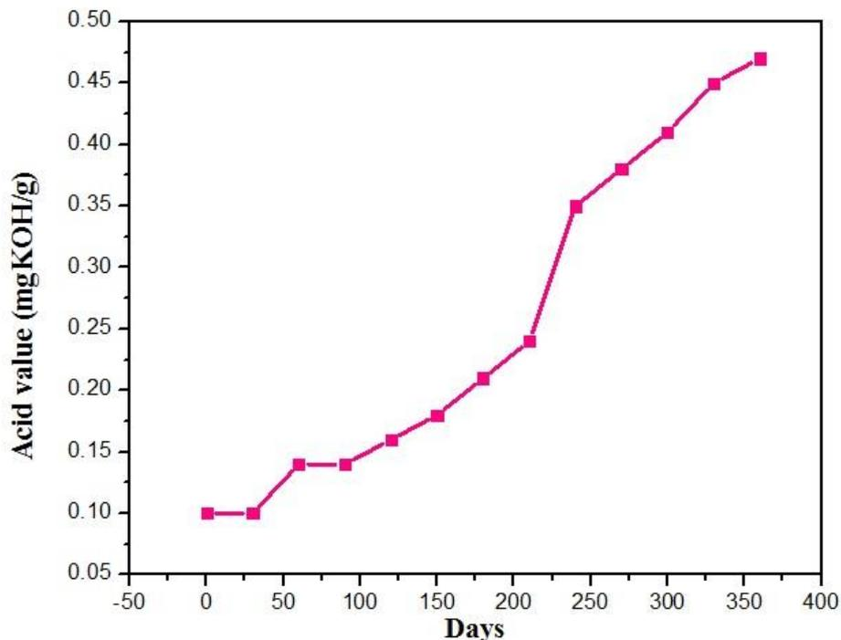
Figure 6. Changes in acid value of biodiesel during storage.
