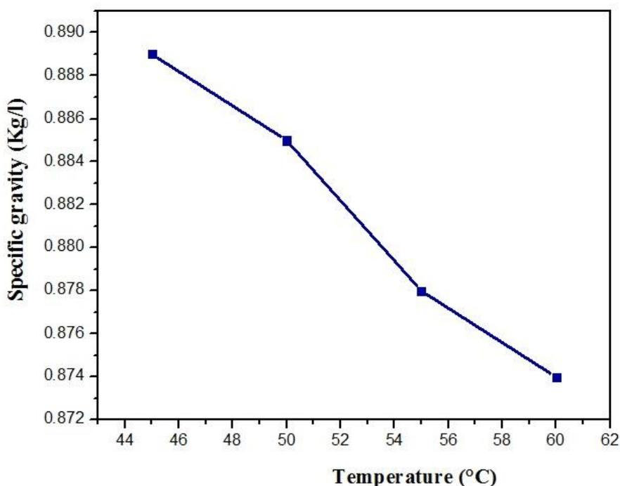
**Figure 2. Effect of specific gravity with respect to temperature**
