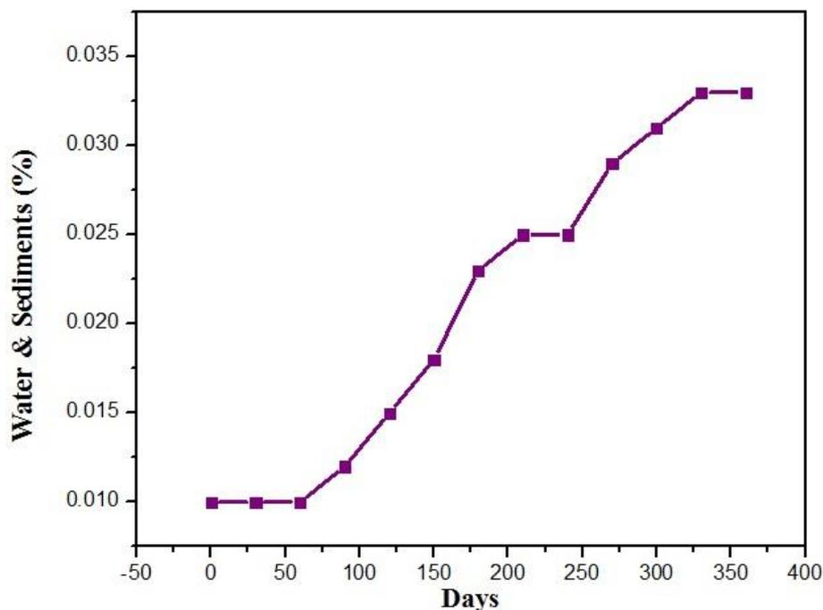
Figure 9. Changes in water & sediments of biodiesel during storage.
