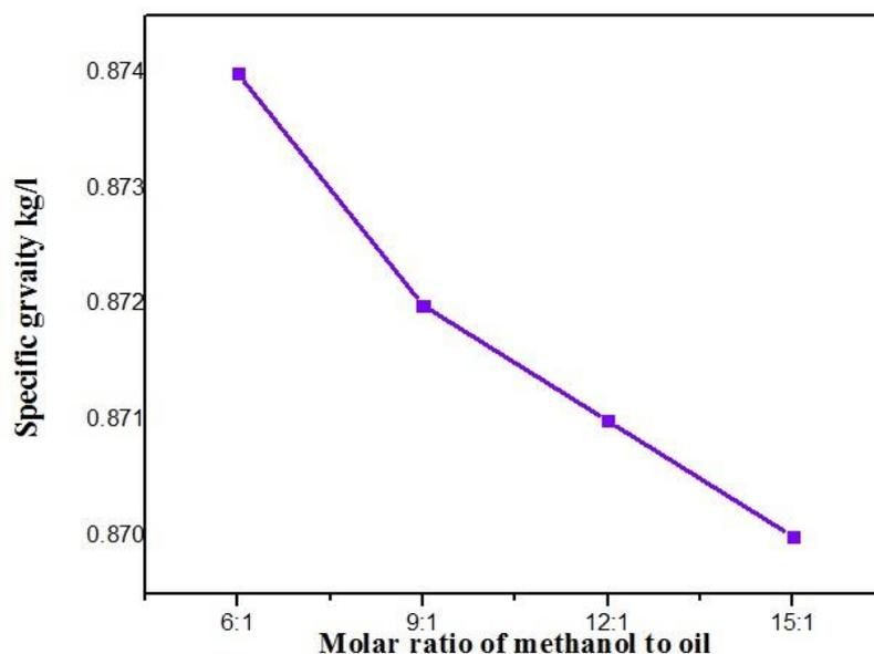
**Figure 1. Effect of specific gravity with respect to molar ratio**
