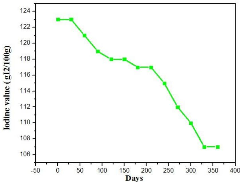
*Figure 8. Changes in iodine value of biodiesel during storage.*
