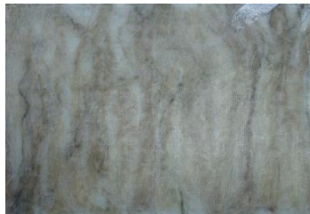
Figure 18: Specimen 200x300 mm before compression
