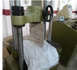
Figure 19: Compression test in universal testing machine
