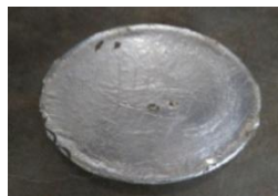
Figure 11: Pattern making for Oval shape E-glass fiber composite specimen
