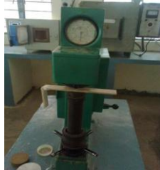
Figure 22: Rockwell hardness testing machine
