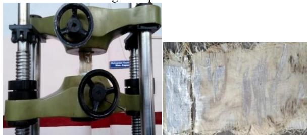
Figure 14: Composite Specimen under universal testing machine Fig.14: Specimen after tensile test
