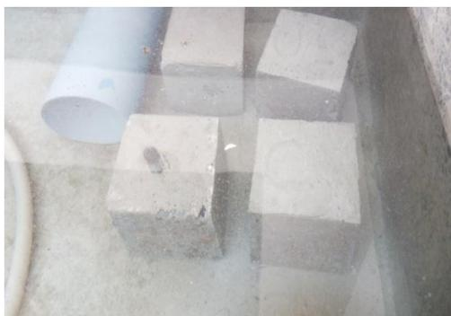
Fig2.3:- Curing in tank
