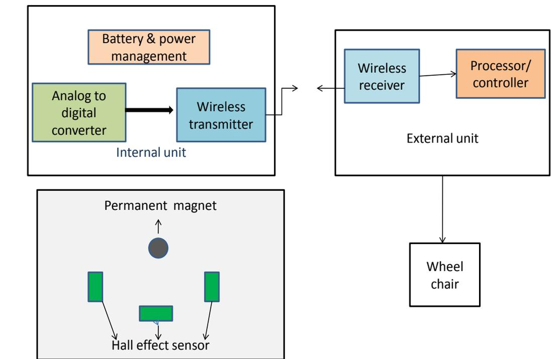
**Figure 2. Block Diagram of Tongue Drive System**
