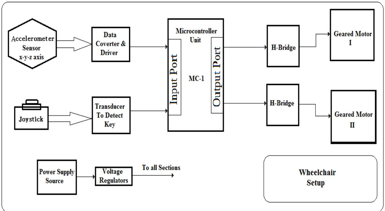
Figure 3. Block diagram of head controlled wheelchair.
