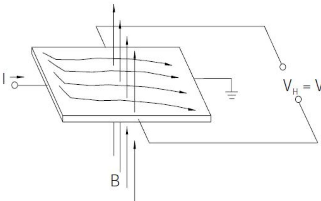
**Figure 5. Hall Effect sensor with Magnetic Field**
