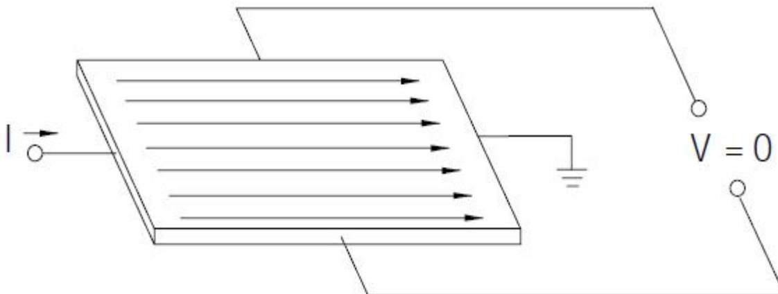
Figure 4. Hall Effect sensor without magnetic field
