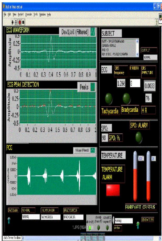
Fig 6: Graphical Analysis of data in LabVIEW
