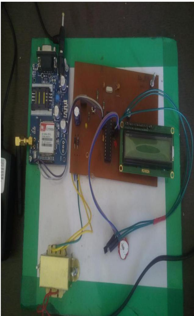
Fig 8:- Hardware of health monitoring system
