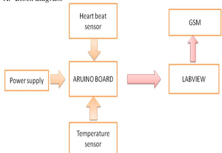
Fig 1: Block diagram of health monitoring system
