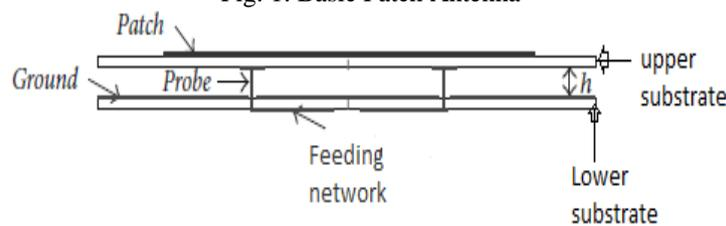
Fig. 2. Layout of Microstrip Patch Antenna
