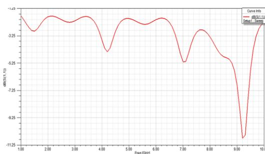
**Fig: 5.a Return loss of basic Patch Antenna**
