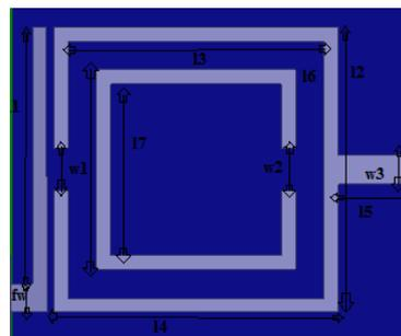
Fig. 3 Structure of Split Ring Resonator
