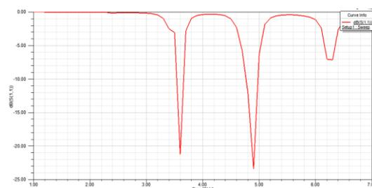
**Fig: 5.b Return Loss of Microstrip Patch Antenna**
