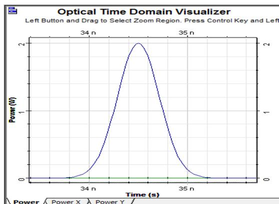
Figure 2. Simulation result for before transmission of signal
