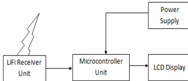
Fig.4 Block Diagram – Receiver Unit
