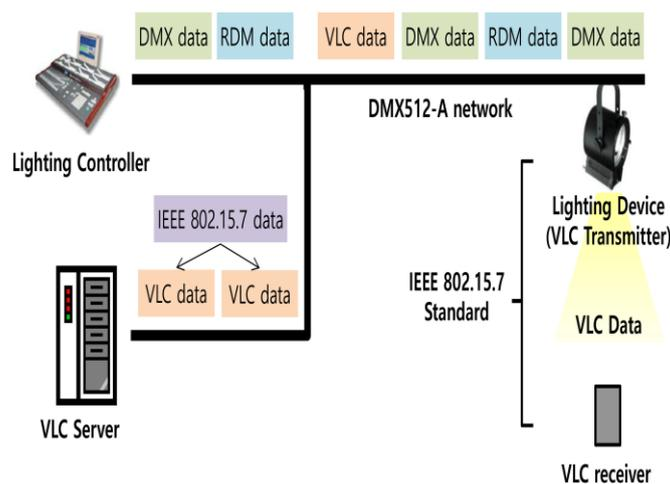
Fig.5 VLC Data Transmission on DMX512-A Network
