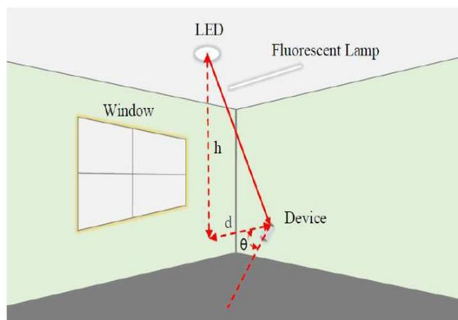
Fig.1 Indoor visible light communication system
