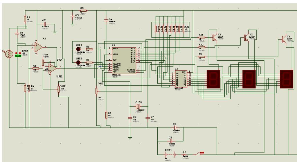
Figure 3. Circuit diagram of heart rate meter
