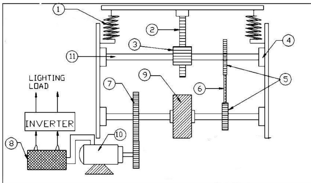
Figure. Rank and Pinion operated Suspension energy generation
