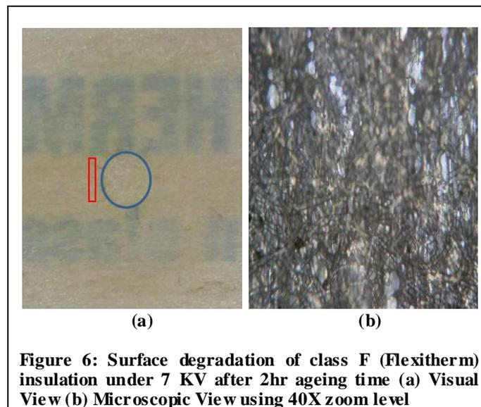
Figure 4 to 8 show the picture of each sample for virgin and aged images of the degraded area on the samples. In this figure circle parts shows the undegraded parts of insulating materials & rectangular area shows the location observed under the microscopic view. The parts (b) of the all figures are images taken using microscope.
