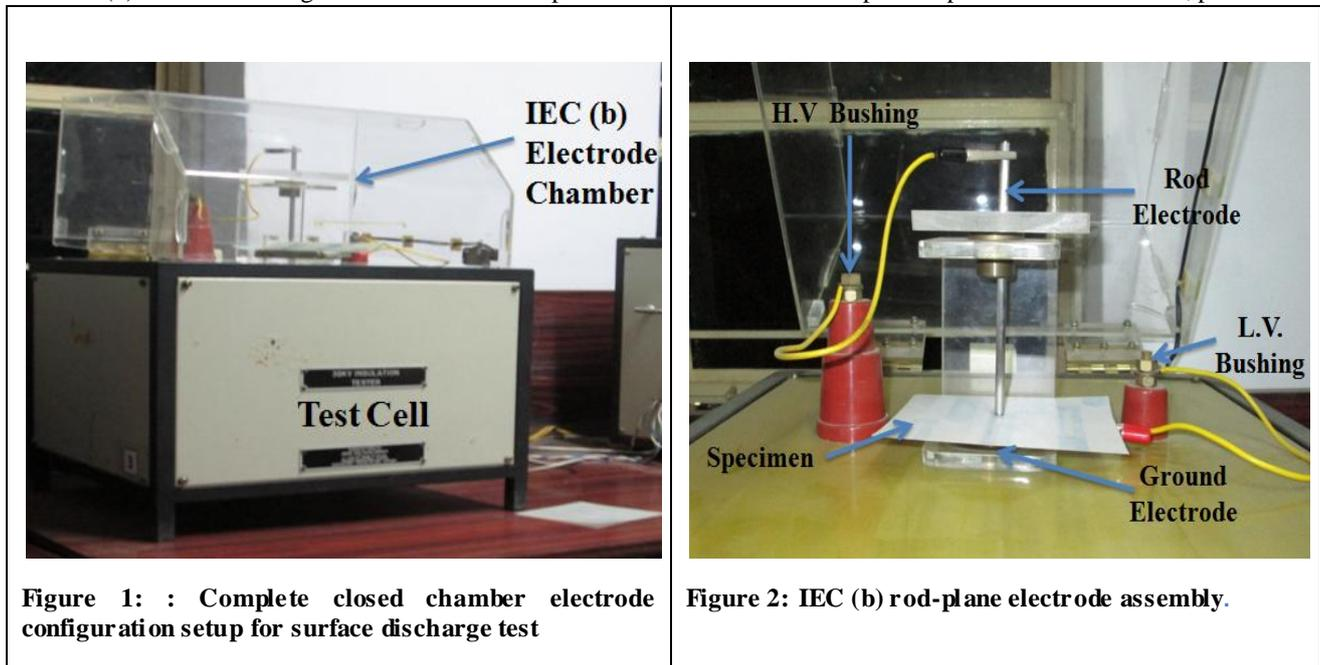
electrode, and closed chamber. The diameter of the rod electrode is 6 mm with radius of curvature 1 mm. The sample was placed in between the rod and plane electrode. Figure 2 shows the IEC (b) rod-plane electrode assembly setup used in the current research.
