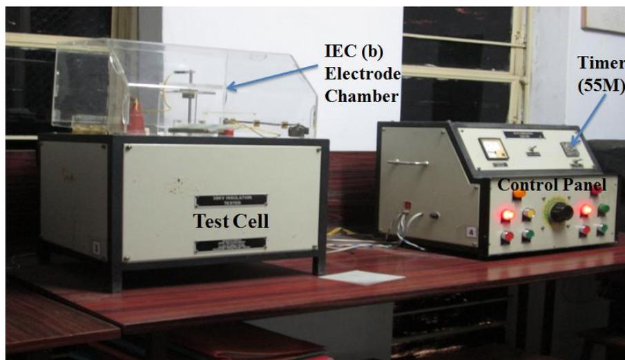
Figure 3: Experimental setup for surface discharge test
