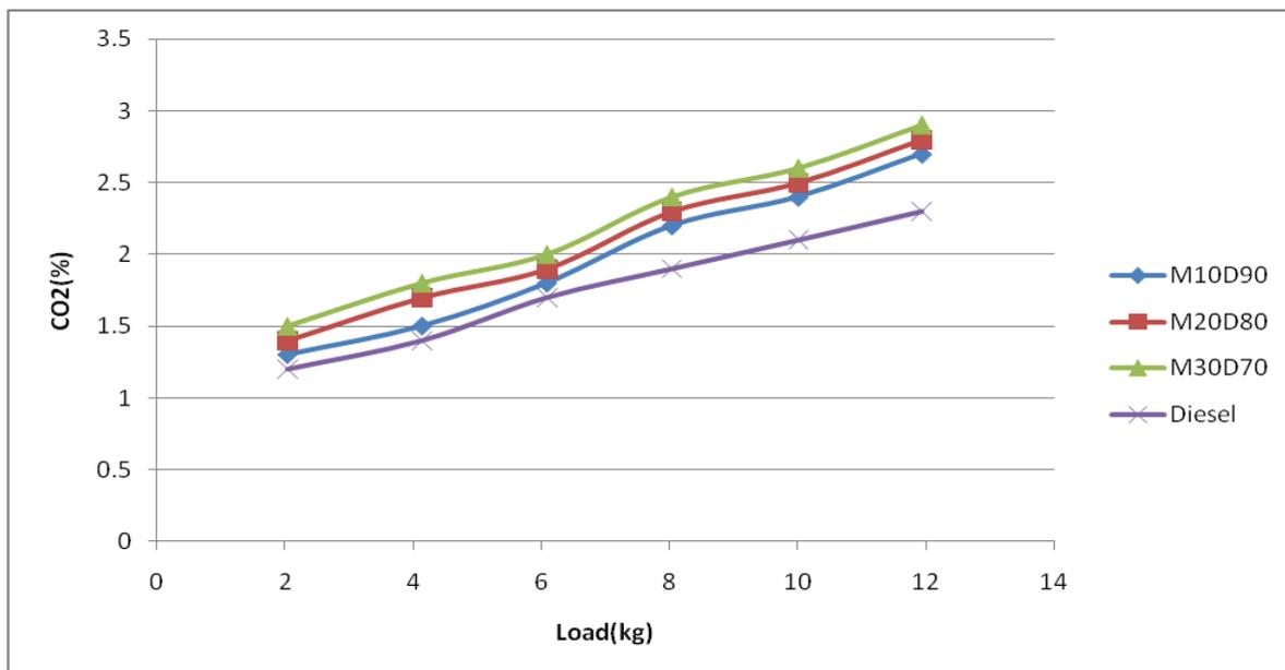
Figure 7:Load v/s CO<sub>2</sub>
