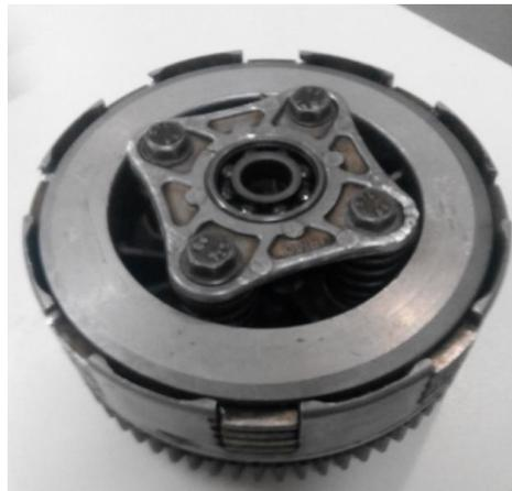
Figure 3. Deep groove ball bearing in clutch assembly
