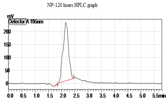
Figure 6: Shows the 120 hour reading of Hydrolysis process using HPLC
