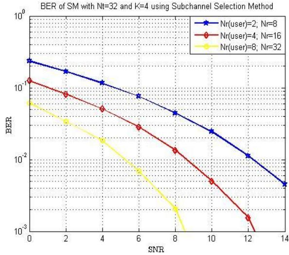
Fig 3.2: BER performance of Massive MIMO System using Subchannel Selection Method
