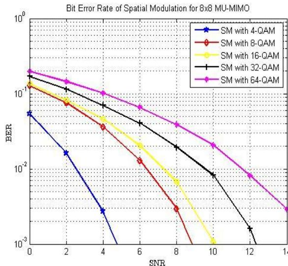
Fig 3.1: BER performance for 8x8 MU-MIMO using MMSE Precoding
