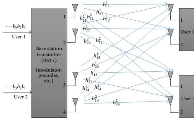
Figure 2.2: SM for Massive MIMO system with  $K_r = 2$ ,  $N_t = 4$ , and  $N_r = 2$
