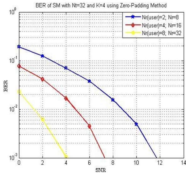
Fig 3.3: BER performance of Massive MIMO System using Zero-Padding Method
