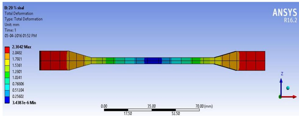
**Figure 3.12 Total deformation of 20% sisal polyester composite**
