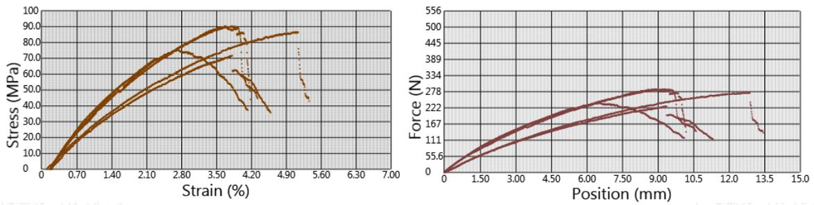
**Figure 3.6. Flexural strength of 20% sisal polyester composite**
