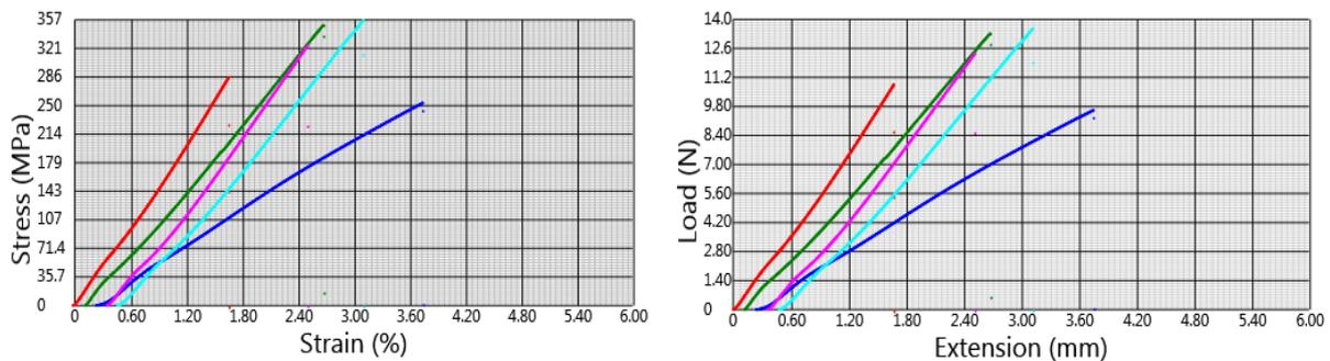
**Figure 3.1. Tensile strength of sisal fibre**
