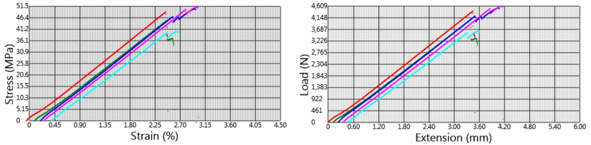
**Figure 3.4. Tensile strength of 20% sisal polyester composite**
