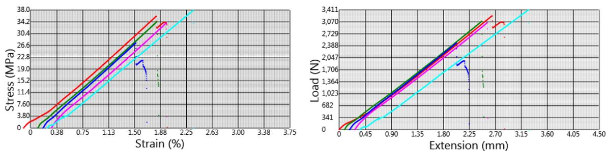
**Figure 3.3. Tensile strength of 10% sisal polyester composite**
