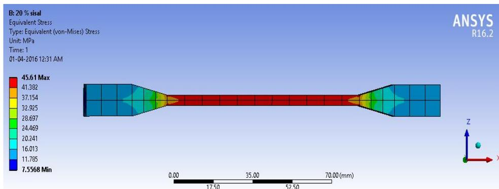
Figure 3.11 Equivalent stress of 20% sisal polyester composite
