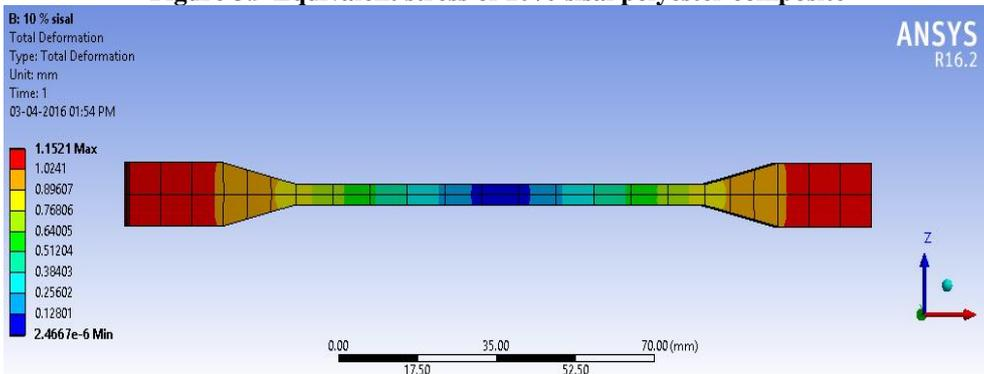
Figure 3.10 Total deformation of 10% sisal polyester composite
