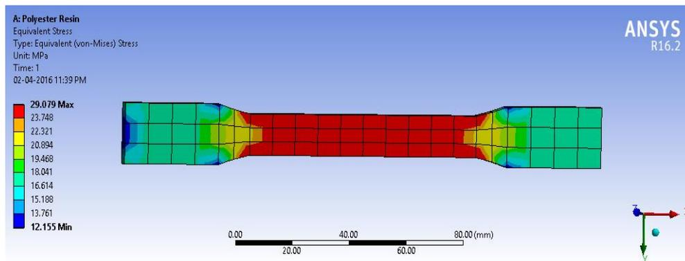
**Figure 3.7 Equivalent stress of polyester resin**
