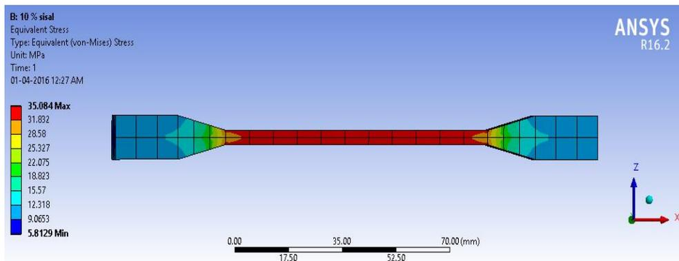
Figure 3.9 Equivalent stress of 10% sisal polyester composite
