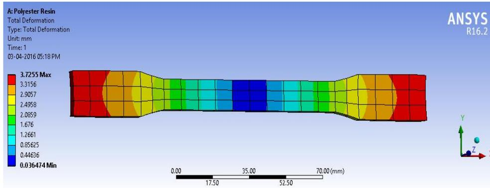
Figure 3.8 Total deformation of polyester resin
