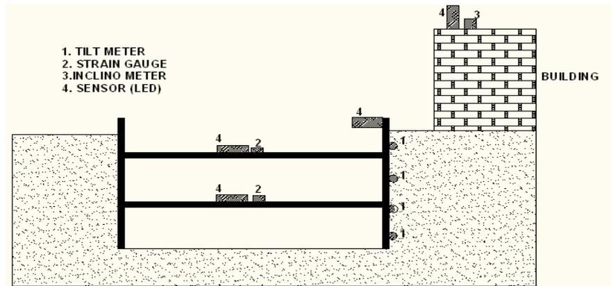
Fig 2 Details of the instrumentation and sensor location
