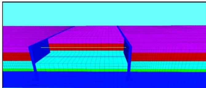
Fig 8: Installation of second strut at 5.35m
