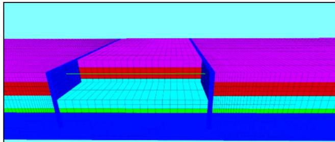
Fig 7: Model after the excavation of 5.5m
