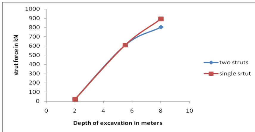
Fig 11: Variataion strut force with depth of excavation
