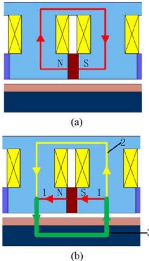
**Figure 5. Flux flow: (a) excitation windings without excitation current and (b) excitation windings with excitation current.**
