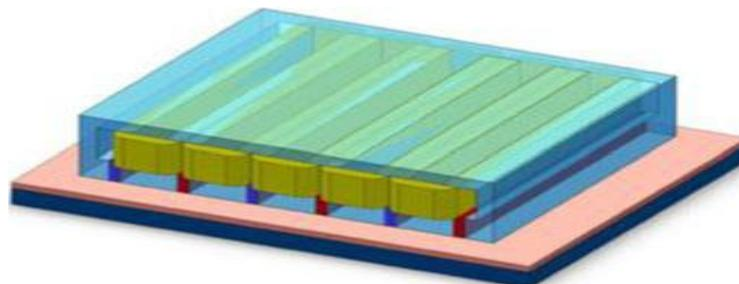
*Figure 2. Three dimensional view of eddy current brake.*
