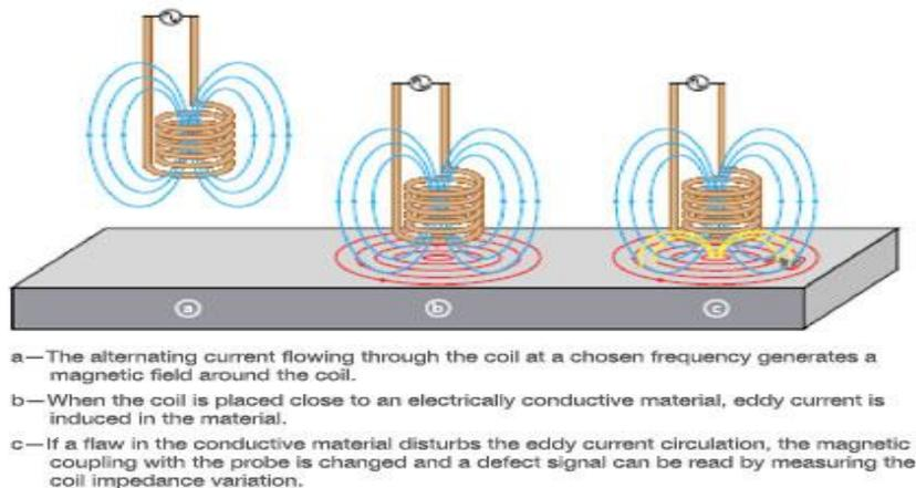
Figure 1. Eddy current produced in a conductor
