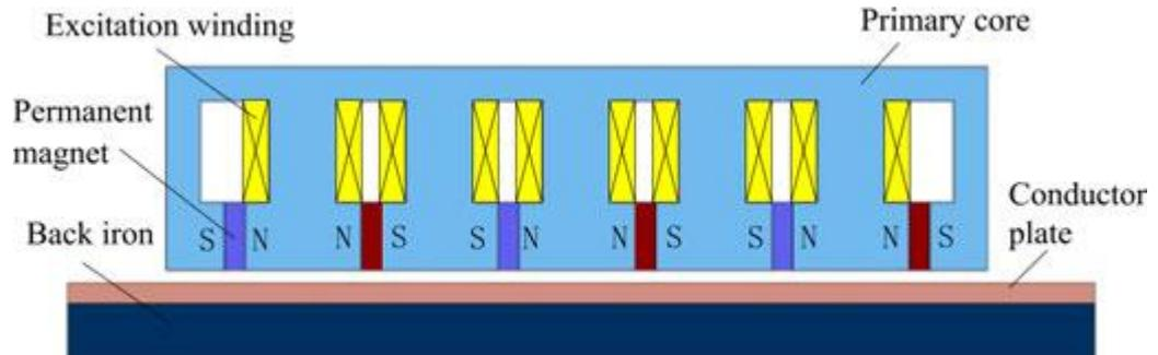
**Figure 4. Side view of hybrid excitation linear eddy current brake.**
