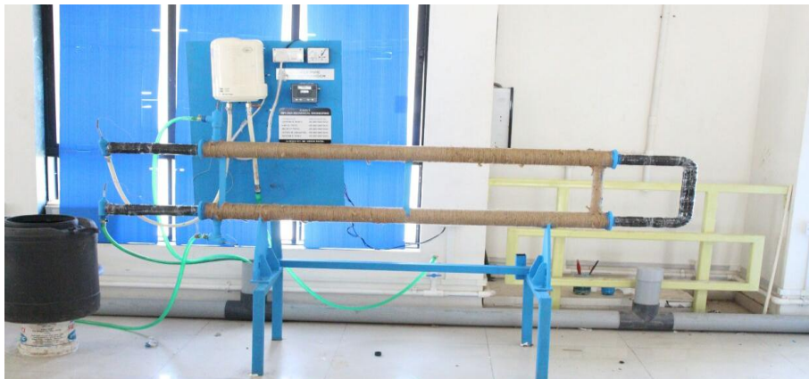
Fig. 1.1 Working Setup of Double pipe heat exchanger
