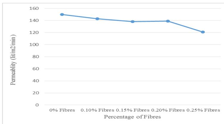
Figure 5.17 shows summarized results on relation between percentage fibres addition in concrete mix and permeability (lit/m<sup>2</sup>/min) after 28day curing.
