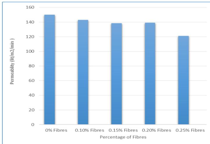
Figure 5.18: Permeability test results after 28days curing
