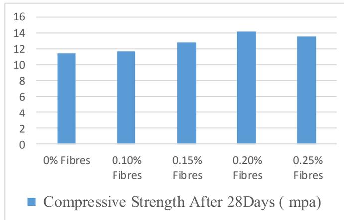
Figure: 5.4: compressive strength on 28 day Curing
