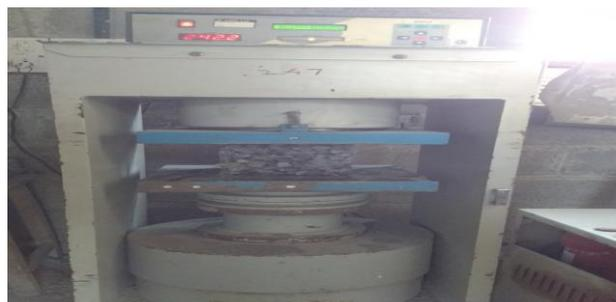
Figure 2.4 Concrete Specimens Testing
