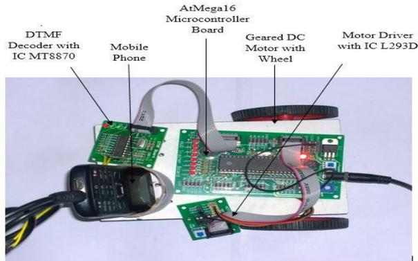
*Figure 2 Shows working model of proposed system*
