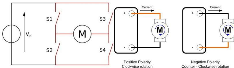
Figure 3.3 Shows H-Bridge circuit Figure 3.4 Shows working of DC motor
