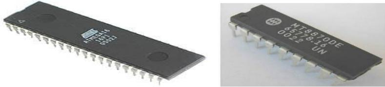
Figure 3.1 Shows Atmega16 Microcontroller Figure 3.2 Shows DTMF decoder IC MT8870
