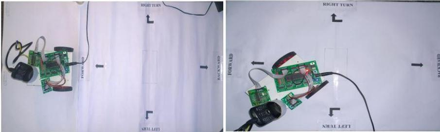
Figure 4.1 shows forward motion when key 2 pressed. Figure 4.2 shows Left turn when key 4 pressed.
