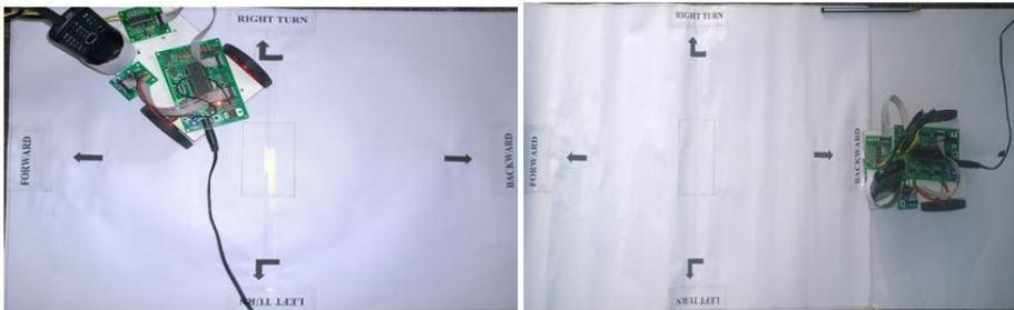
Figure 4.3 shows Right turn when key 6 Pressed. Figure 4.4 shows backward motion when key 8 pressed.
