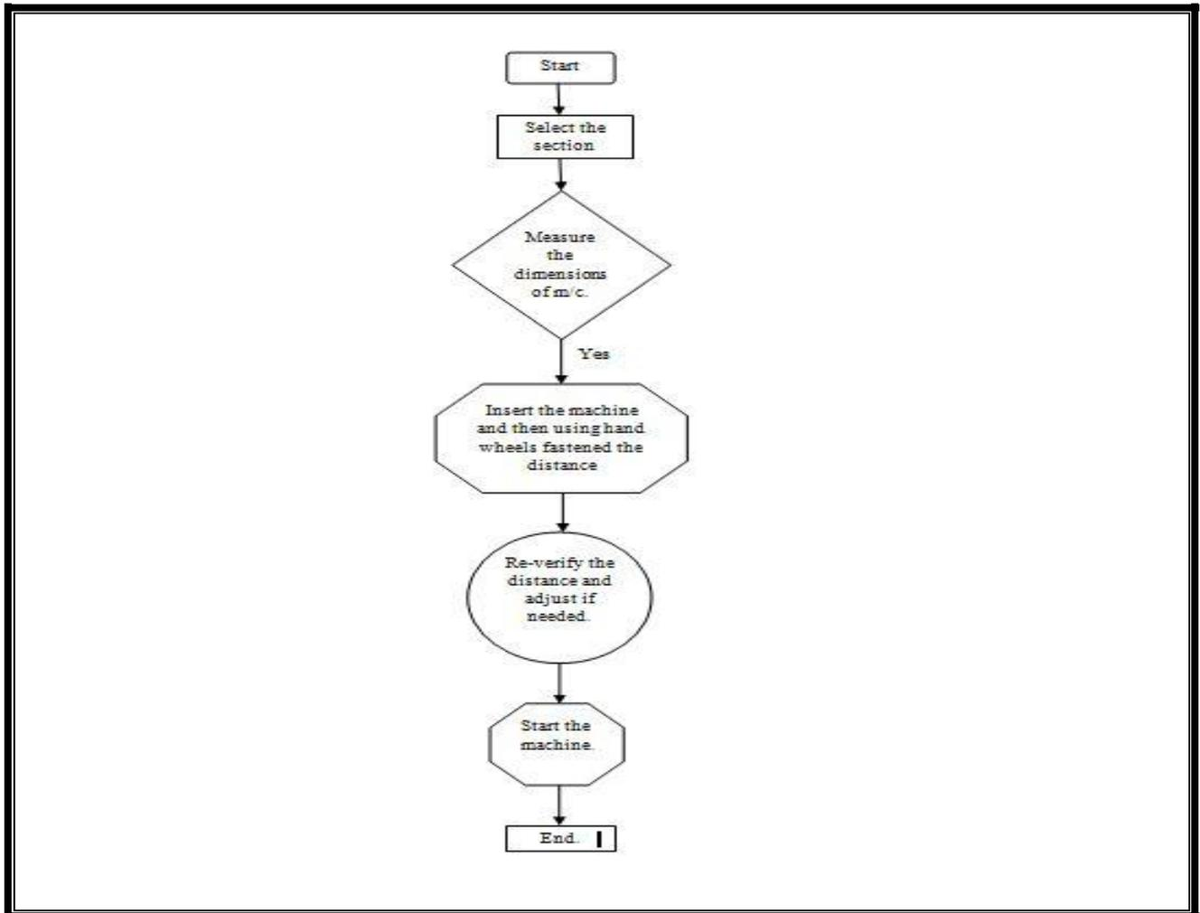
Figure 6: Flow Chart for Assembly of robots for varying Sections
