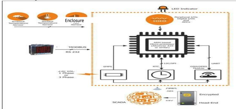
**Figure 4. System architecture of the TMU**
