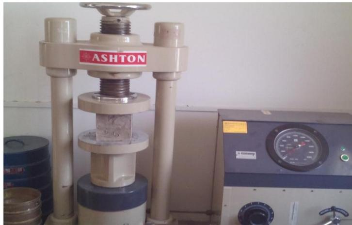
**Fig.6 Compression Test on cubes**
