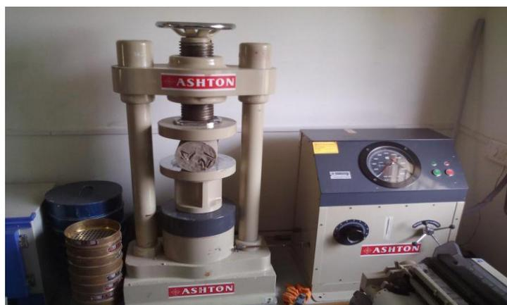
**Fig.7 Testing on cylinder**
