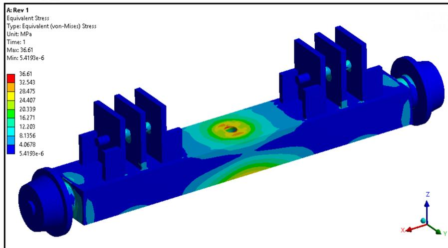
Figure 4.7 Equivalent Stresses MPa
