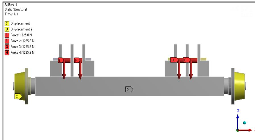
Figure 4.4 Loading & Boundary Conditions
