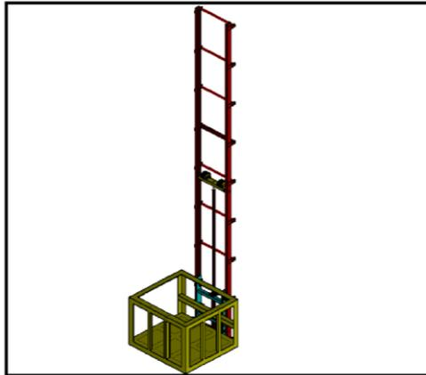
Figure 4.2 Solid work Model Goods Lift
