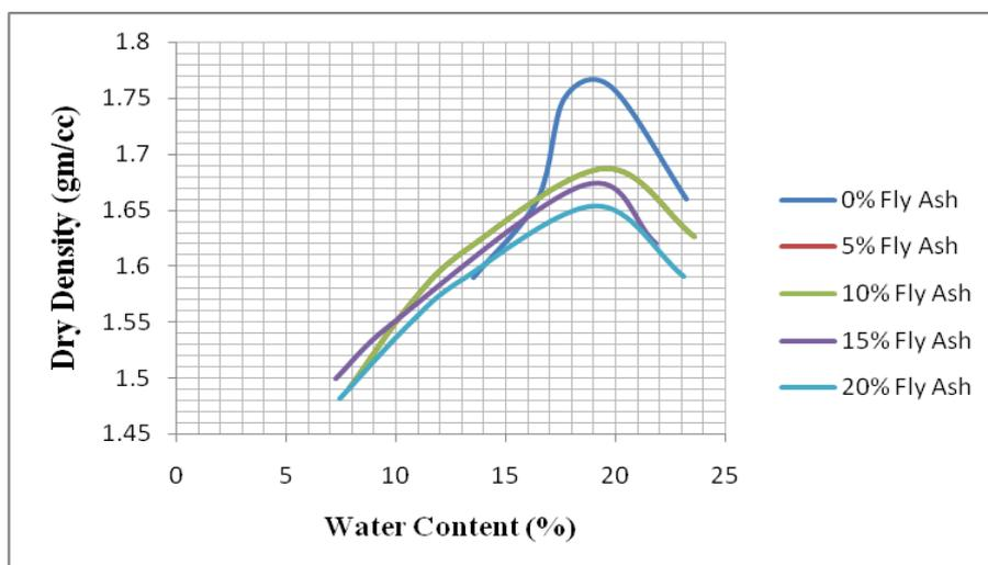
Figure 2 Compaction curves (0.50% Glass Fibre)
