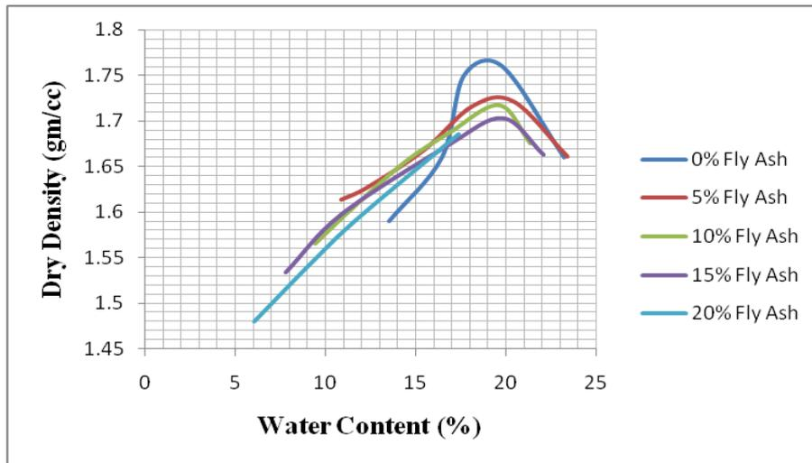
Figure 1 Compaction curves (0.25% Glass Fibre)
