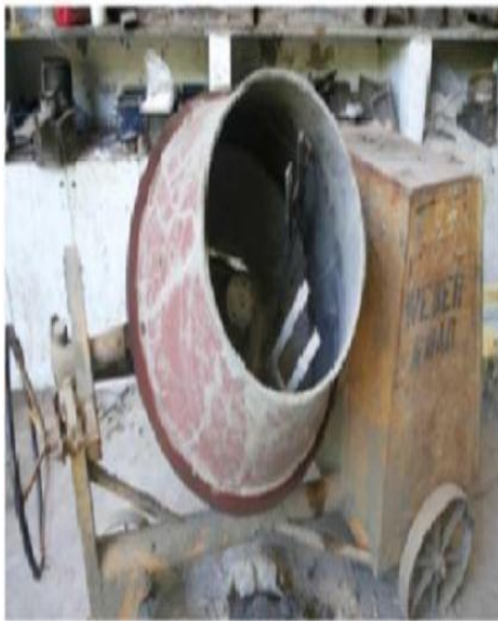
Figure:2 Mixture used for casting of concrete
