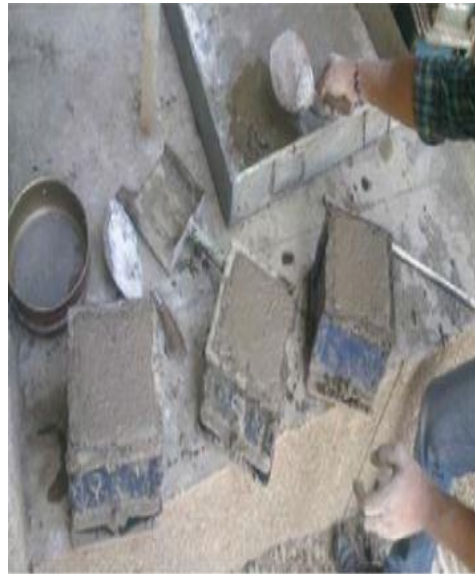
Figure:3 Geopolymer Cubes after casting
