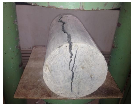
Figure-14 Failure in fibre reinforced specimen
