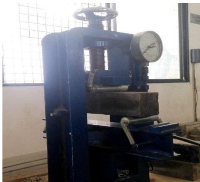
Figure-7 Flexural strength test
