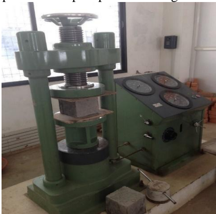
Figure-5 Compressive strength test
