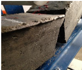
Figure-16 Failure in normal specimen
