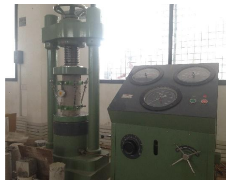
Figure-8 Test for modulus of elasticity
