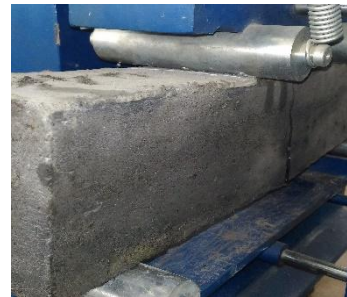
Figure-17 Failure in fibre reinforced specimen
