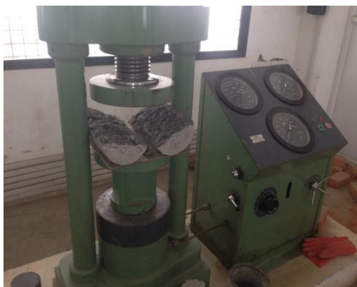
Figure-13 Failure in normal specimen
