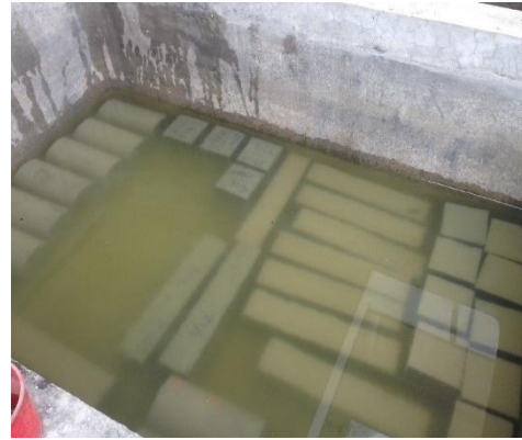
Figure-4 Specimens under curing
