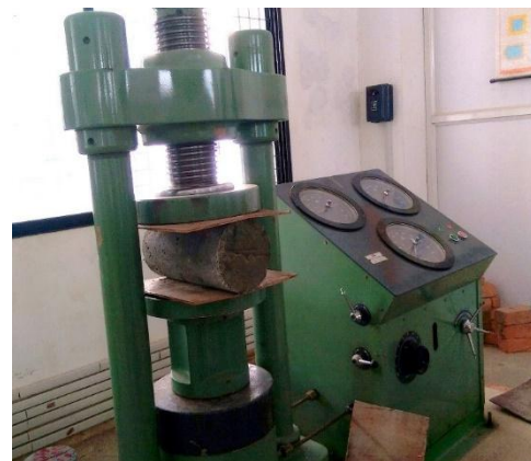
Figure-6 Split tensile strength test
