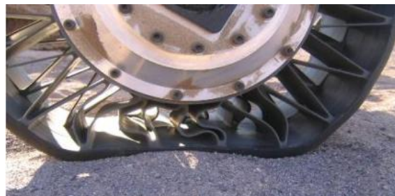
Fig. 5. An ATHLETE Tweel Shown Deforming Over Uneven Terrain
