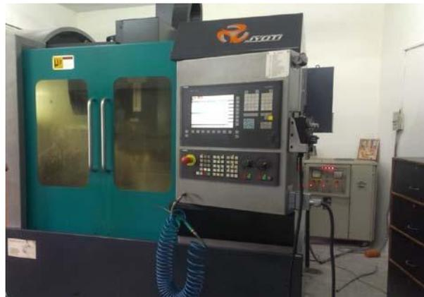
**Figure 2.1. Vertical CNC Milling Machine.**
