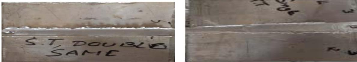
Figure 2.3 Samples of FSW Produced In Final Experimentation
