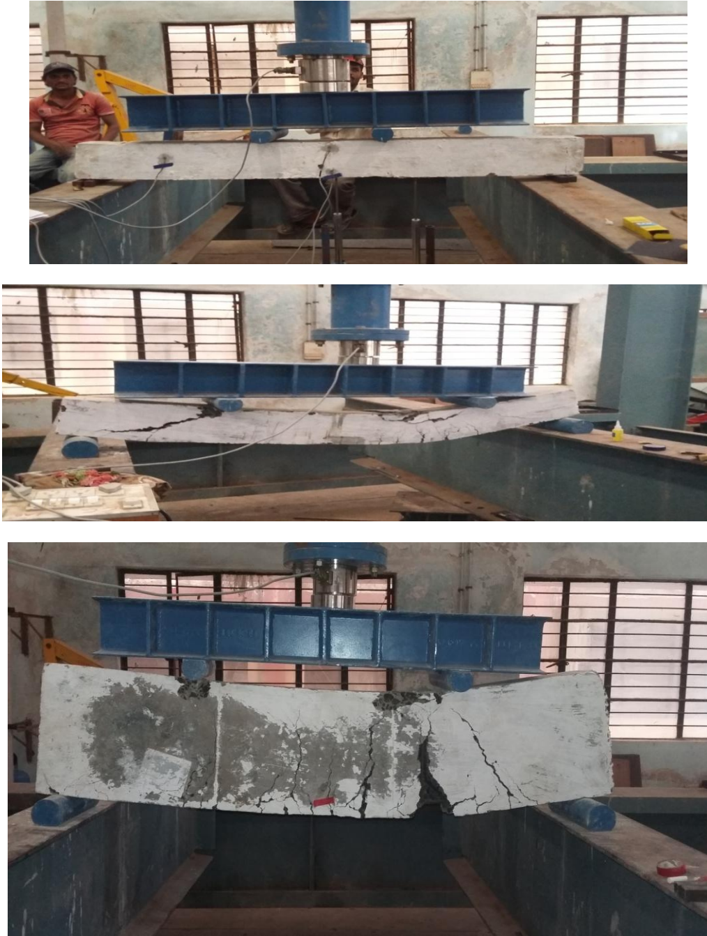
Plate 3 : Testing of beams under the servo Hydraulic Loading frame
