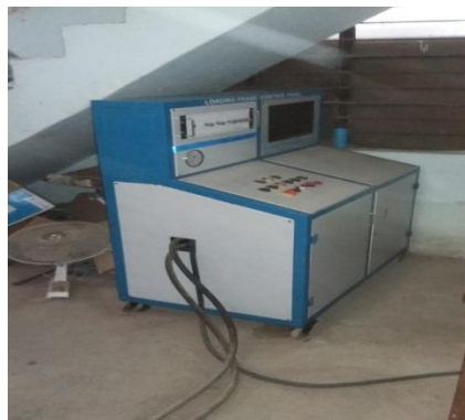
Controller Unit of Loading Frame
