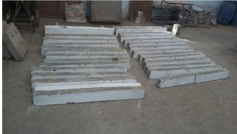
Plate 2: Curing of the Geopolymer concrete
