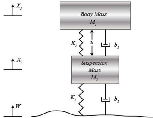
Figure: (i) Passive Suspension System
