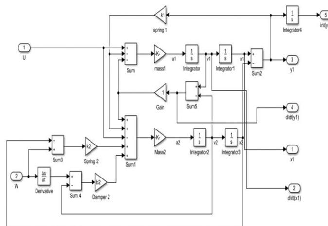
Figure: (iii) Subsystem of Active Suspension System
