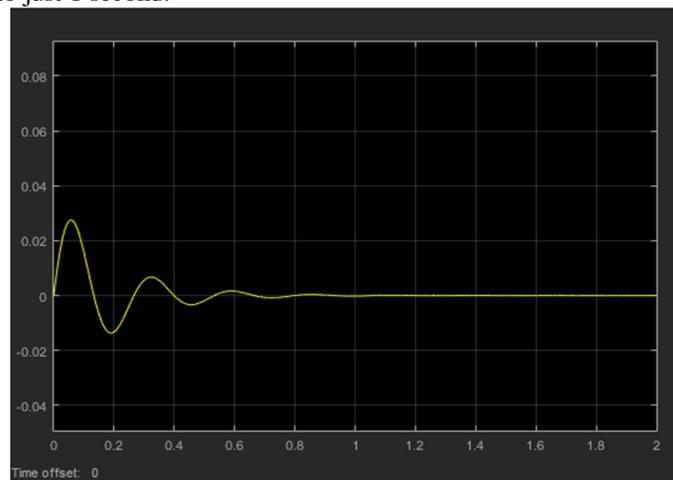
**Graph: (iii) Car body displacement for 10 cm step input for active system**
