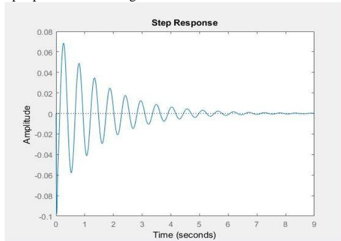
**Graph: (i) Car body displacement for 10cm step input for passive system**
