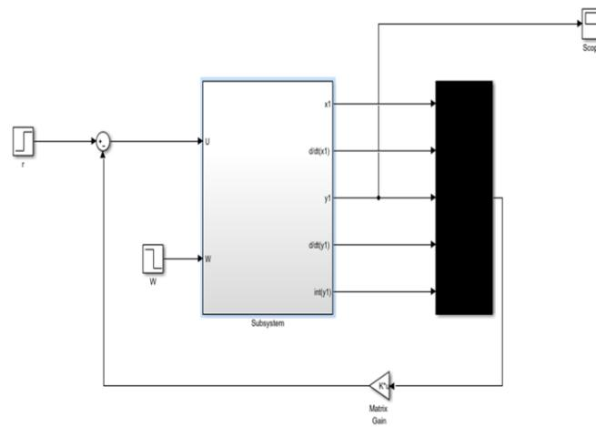
Figure: (ii) MATLAB model of Active Suspension System
