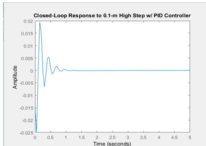
**Graph: (ii) Close loop response to 10 cm high step w/ PID controller**
