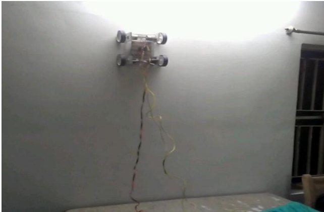
Figure 3. Robot on vertical wall surface
