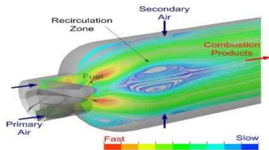
"Fig. 5" Combustion streamlines
