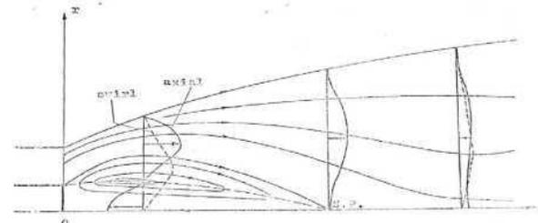
"Fig. 7" Typical profiles of axial and swirl velocity components in a strongly swirling flow
