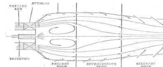
"Fig. 1" Air flow pattern in a conventional combustion chamber
