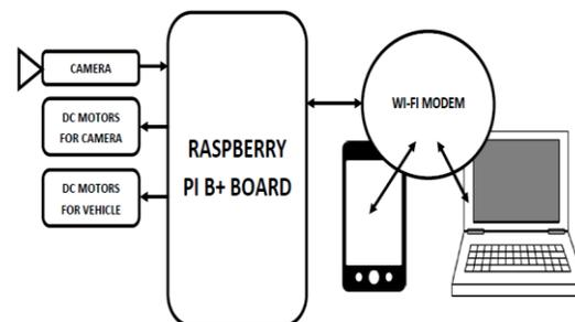
Figure 1: Proposed Block Diagram of System
