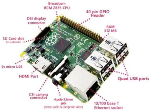
Figure 2: Raspberry Pi B+ Board
