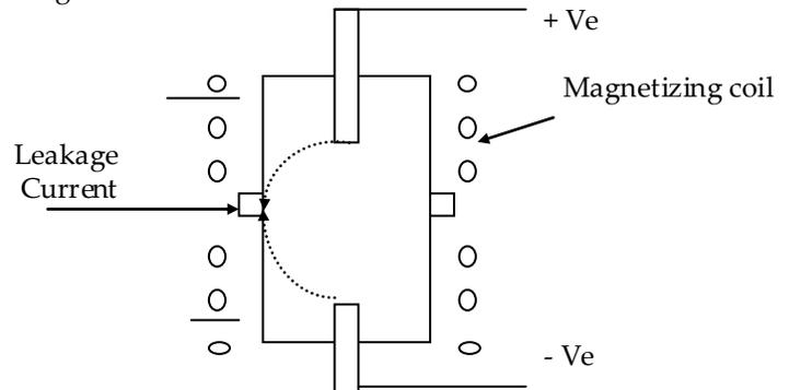
In this system, the open contacts of VI bottle are subjected to high Voltage DC supply to establish the capacitance between two contacts.
