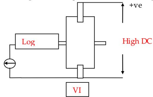
In this method, the high DC voltage [1.2 RATED] is applied across the open contacts of VI and the shielding electrode is kept at ground potential as a Reference voltage and the leakage current is measured by using Logarithmic amplifiers since the current is in neno- amperes.
