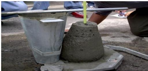
Fig-6: Slump of fresh concrete measured.
