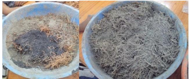
**Fig-4:** Cement mixed with Rice-husk ash and COIR fiber
