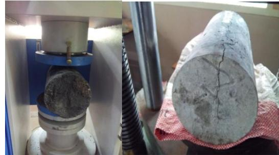
**Fig-8:** Tensile strength of concrete cylinder and failure pattern
