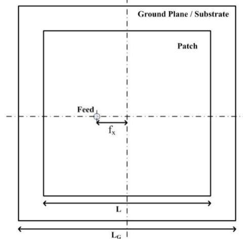
**Fig.2. Conventional Patch Antenna**
