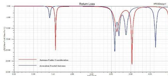
Fig.5. Comparison of Return Loss plots of both conventional antenna and Antenna with Jerusalem Slots
