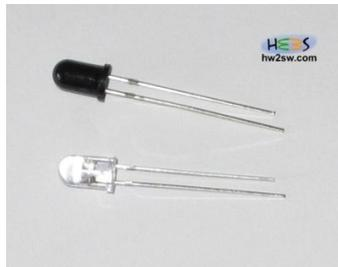
To detect car, Infrared TX/RX is used and simultaneously gives signal to PLC to trigger the respective compartment operation.
