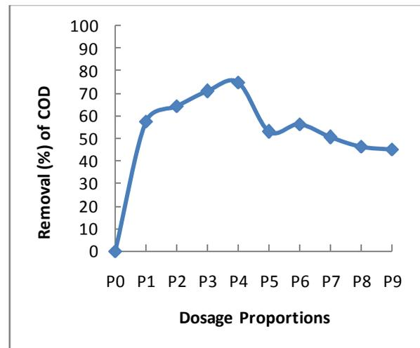
Figure 7. Removal (%) Of COD With Various Dosage Proportions of Sp:  $(Al_2(SO_4)_3)$ .
