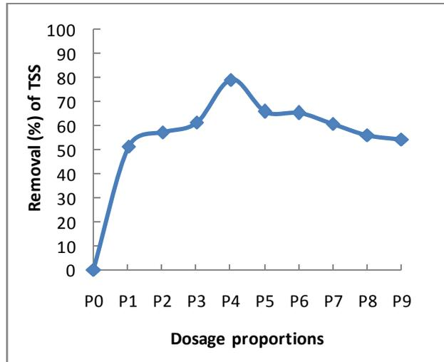
Figure 5. Removal (%) Of TSS With Various Dosage Proportions of Sp:  $(Al_2(SO_4)_3)$ .
