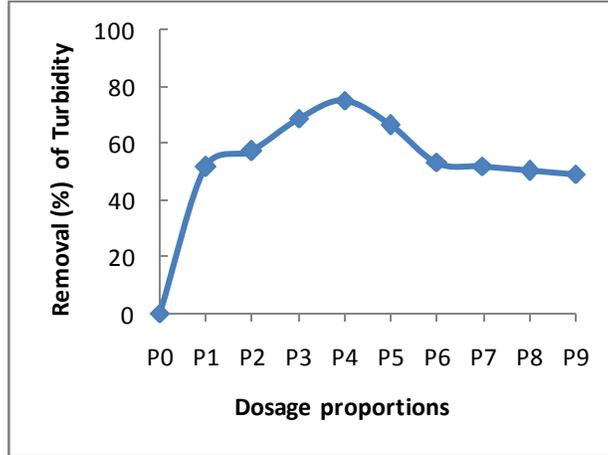
Figure 3. Removal (%) Of Turbidity With Various Dosage Proportions of Sp:  $(Al_2(SO_4)_3)$ .
