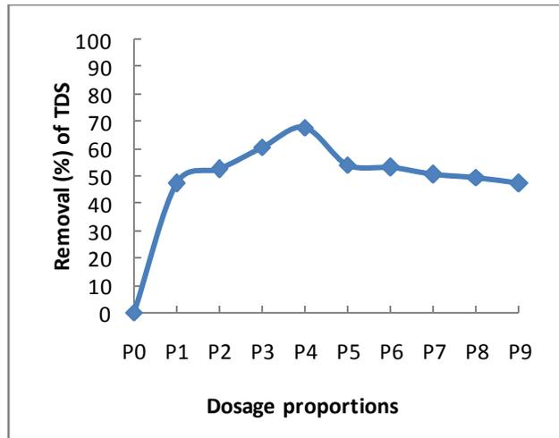
Figure 4. Removal (%) Of TDS With Various Dosage Proportions of Sp:  $(Al_2(SO_4)_3)$ .
