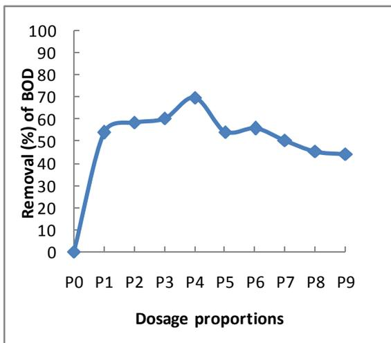
Figure 6. Removal (%) Of BOD With Various Dosage Proportions of Sp:  $(Al_2(SO_4)_3)$ .
