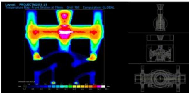
Figure 6. Temperature map at front section at 79 mm
