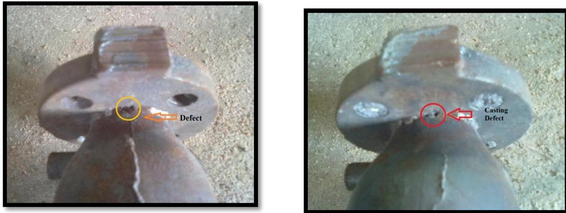
*Figure 1. Defective Globe Valve*
