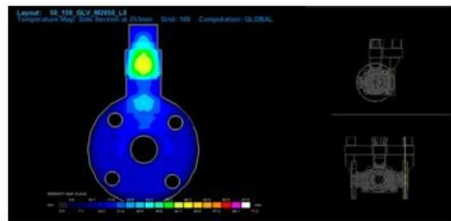
**Figure 13. Temperature map at side section at 253 mm**
