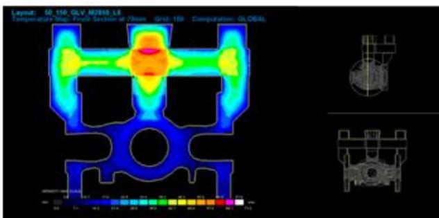
**Figure 12. Temperature map at front section at 78 mm**
