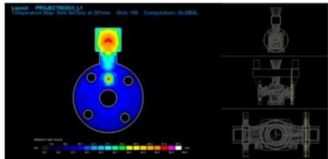
Figure 7. Temperature map at side section at 261 mm
