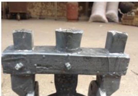
**Figure 15. Modified gating system part**
