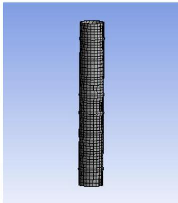
Fig. 3 Meshing of CHS sections
