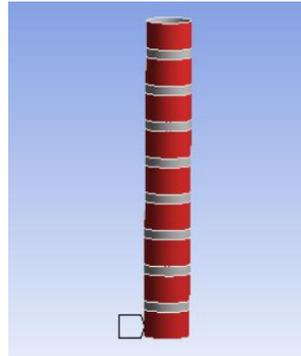
Fig.2. CFRP wrapped specimen
