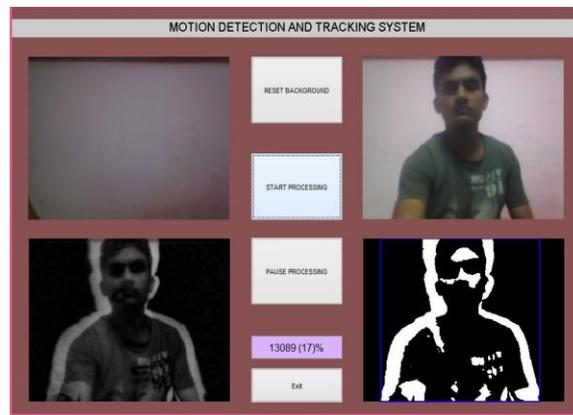
Fig. 4 Human is detected (i.e Blob is detected)
