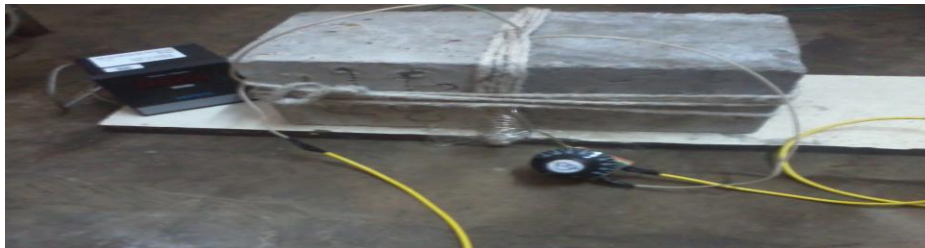
“Figure 8: putting j-type thermocouple at outer surface”
